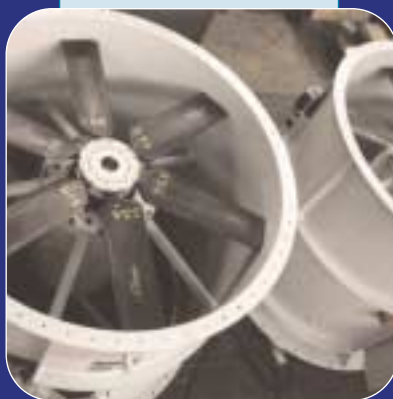
Top: E-series fan in a 32 ft. cooling tower
